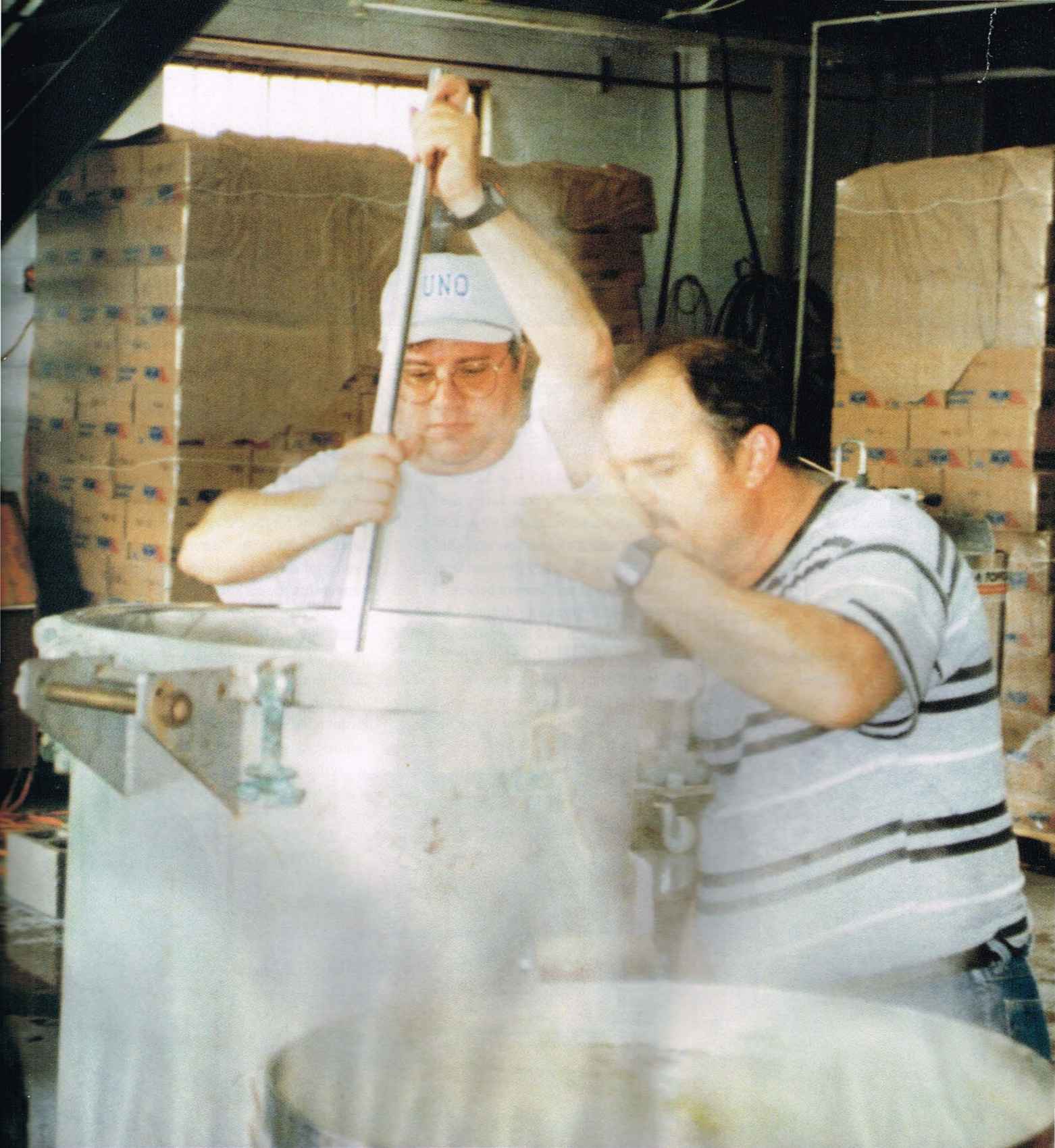
Denis Finigan helps Doug Lindley by stirring the wort. Propane burners heated the 50- and 60-gallon brewpots for the boil. The shorter brewpot used to be part of a commercial stainless-steel washing machine.
