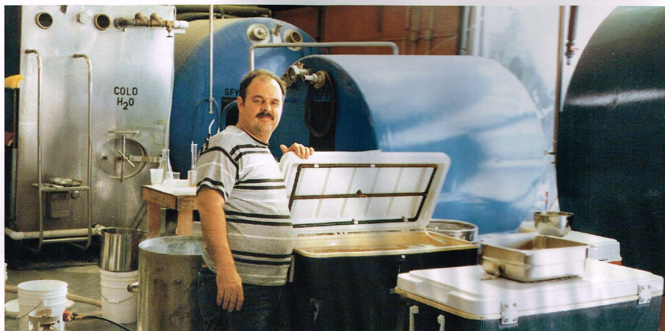
Doug shows the inside of a lauter tun lid. The perforated copper pipe is connected to a stainless-steel pan attached to the top of the former ice chest.
